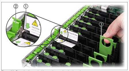
Figure 28: Deactivating, unlocking and removing the board
